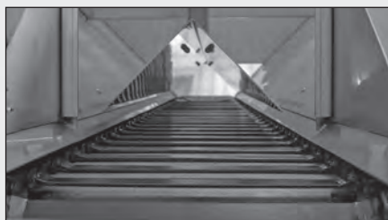
24" wide conveyor chain with 3/8" bars
