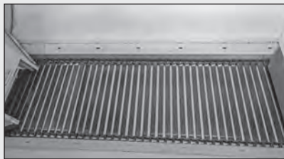
30.25" wide conveyor with 1/2" bars
